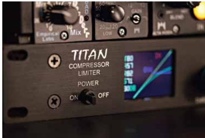
The 1U front panel includes a bright, color LCD screen that displays numeric values for five adjacent "Cranesong green" knobs: Threshold, Attack, Release, Shape and Gain.
